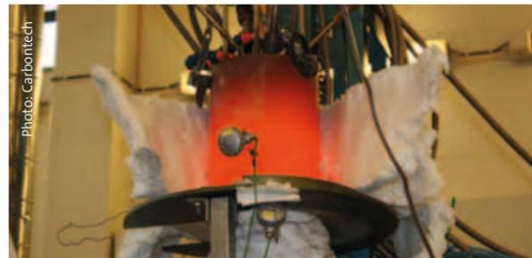
Pilot facility for production of carbon nanoparticles.
